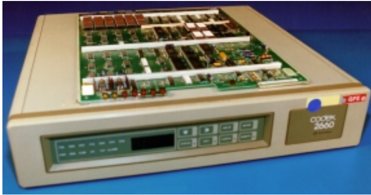
Figure 5. A Codex 2660 Four-wire, Leased-line Modem that Employed Trellis Coding and 256-QAM to Attain a Transmission Rate of 16800 b/s
