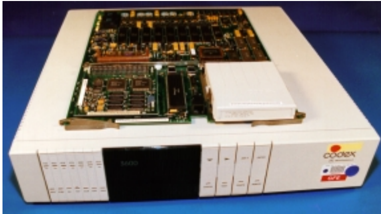
Figure 7. A Codex 3600 Modem that Used a Higher Symbol Rate and Trellis Precoding to Attain Transmission Rates of 24000 b/s
